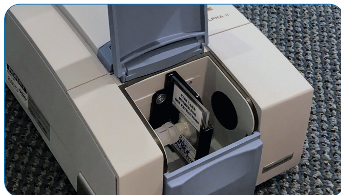
Fig. 2: Oil membrane mountend inside ALPHA II FTIR spectrometer.
