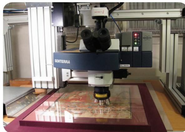
Figure 1: Raman microscope SENTERRA II mounted on a
