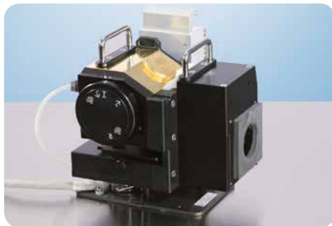
Fig. 1: Gold coated integration sphere A562 for diffuse reflectance measurements with two alternative openings used as sample position or specular light trap (top or bottom). The whole sphere including detector can easily be inserted into or removed from the FT-IR sample compartment such that the spectrometer can also be used for further applications.
