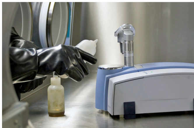
Figure 6: ALPHA spectrometer inside a glovebox.
