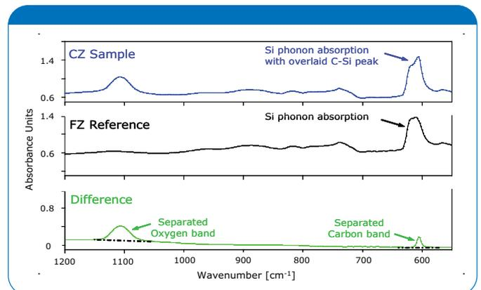
Fig. 3: Room temperature absorbance spectra of a 2 mm CZ silicon sample, a 2 mm FZ silicon sample and the resulting difference spectrum. Evaluation with OPUS/SEMI results in a Carbon concentration of  $3.1 \cdot 10^{17}/\text{cm}^3$  (6.2ppma) and an Oxygen concentration of  $1.0 \cdot 10^{19}/\text{cm}^3$  (20.1ppma). The spectra were measured using a VERTEX FTIR spectrometer with DTGS detector, KBr beamsplitter and a resolution of  $4\text{ cm}^{-1}$ .
