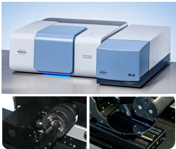
Fig. 1: Top: PLII module adapted to INVENIO R research FTIR spectrometer. Lower left hand side: standard glass objective with vertical sample mount. Lower right hand side: mirror objective and X-Y mapping stage for convenient horizontal sample positioning.
