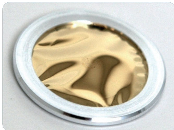
Figure 5: Gold filter for the isolation of particles from liquid formulations.
