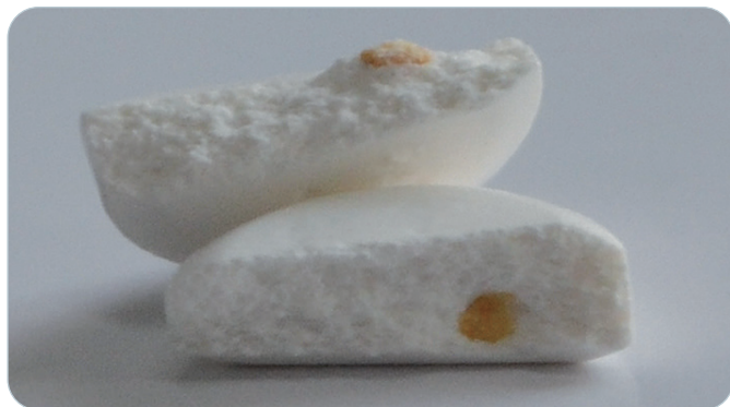
Figure 2: Pharmaceutical tablet with contamination (yellow).
