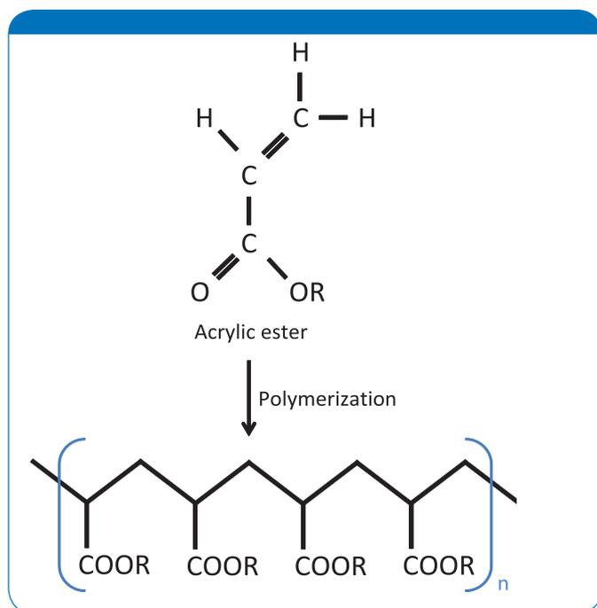
Fig.2: Basic reaction scheme of an acrylic varnish.
