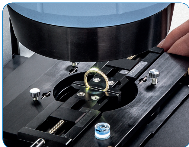
Figure 9: Diamond ring fixed in the sample holder vice on the LUMOS II stage.
