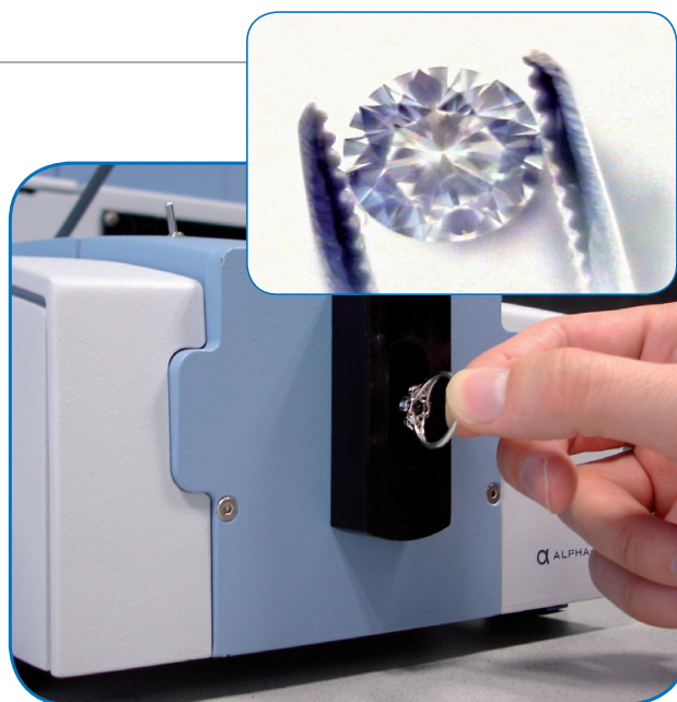
Figure 7: ALPHA II with front reflection module. Inset: Picture of a diamond taken with the integrated camera.
